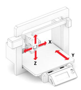
"Cartesian 3D printer is named after the XYZ dimensional coordinate system. The extruder moves in two directions (X and Z), while the print bed moves along the Y-axis. It also means that the print bed is usually square- or rectangle-shaped. Original Prusa i3 MK3S is a cartesian printer." (1)
