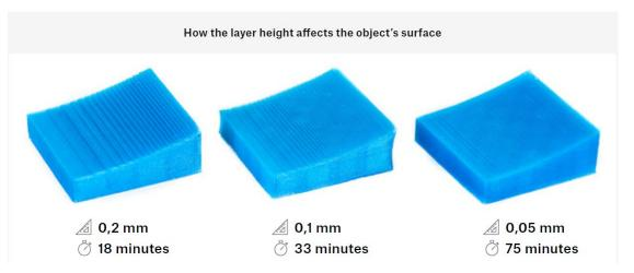
"Layer height – sometimes also called the "Z-axis resolution" has a major impact on both print times and overall surface finish of the printed object. Higher values lead to faster prints and more visible layers on the surface of the object. This effect is especially prominent on surfaces that are nearly parallel to the print bed. Most of the time, layer heights of 0.15mm - 0.20 mm are preferred."(1)
