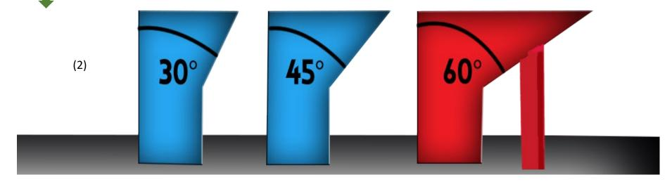
"Overhang angles are extremely important to take into consideration when designing a part to be 3D printed. Without understanding how support structures work, it is easy to think that any structure can be easily printed with a clean surface quality.
